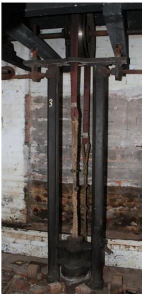
Stamping is carried out using a piece of machinery known as a “drop (or forge) stamp.” This machinery is still in use today within the Jewellery Quarter. A large heavy stamp would be dropped from a height onto a sheet of metal to make decorative patterns on the breast plate. The drop stamps at Newmans were powered by an electric motor which drove the line shafting above the machines. The stamps were operated from a pit dug into the floor behind them.
