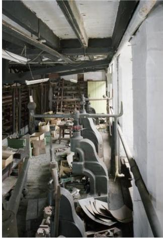
These machines were used to clip off surplus metal around the pressings to form cleanly finished fittings. The fly presses were also used to create smaller stamped items (see the crucifix shape below).
